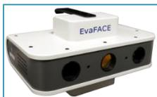
The EvaFACE was later developed to specially address global face 3D analysis at a more affordable cost. Its cameras exhibit a similar resolution and its FOV has a diagonal of 300mm, a lateral resolution of 82 $\mu$ m and a Z resolution of 10 $\mu$ m.
